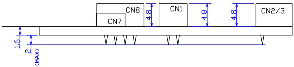
※Tolerance: ±0.3mm except for hole diameter
