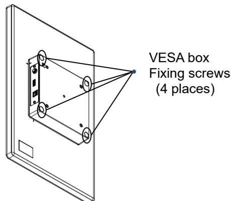
[Caution] Make sure that wires are not trapped between the box and the main unit.
