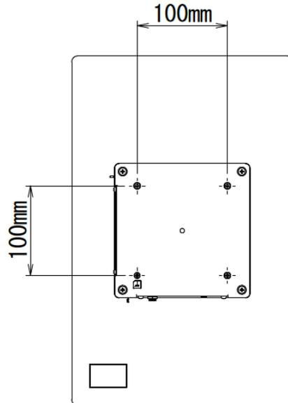
Use M4 screws with tightening torque of 0.7 to 0.8N-m
