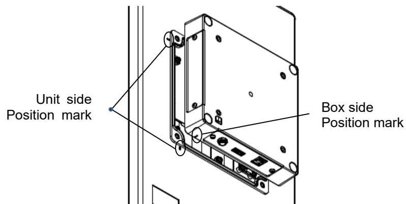
[Caution] Lifting the VESA box too high may break or damage the wires.
