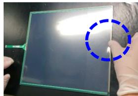
5. Finally, after finishing step 4, slowly apply pressure towards the directions as shown in the picture to attach the whole film and touchscreen surfaces, then remove the protective film on the front side.
