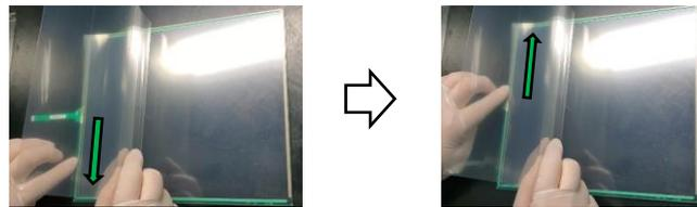
3. To avoid air bubbles, while holding down the short edge that was first attached, peel off the protective film slowly towards the other side of the touchscreen, allowing the anti-virus & anti-bacterial film to be attached to the touchscreen by its weight.
