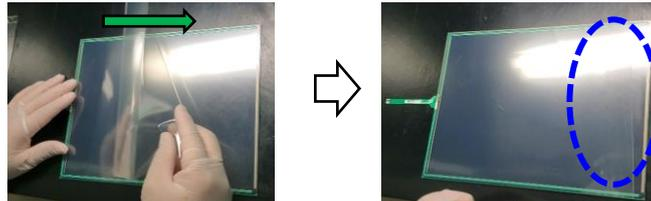
4. Press the center of the unattached area with the thumb as shown in the picture.
