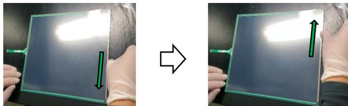
\*\*If the touchscreen is a resistive type, removing the protective film should be done by peeling it off slowly in the horizontal direction, in order to avoid the ITO film from being stressed. If it is peeled off strongly and rapidly in the vertical direction, the ITO film could be distorted.
