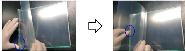
2. After finishing step 1, attach the whole side of the short edge by applying pressure from the center towards the directions as marked in the picture.
