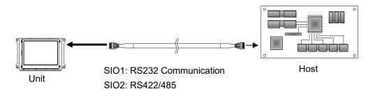
\*Applying Ferrite Core to the communication cable is recommended for noise and static measures.
